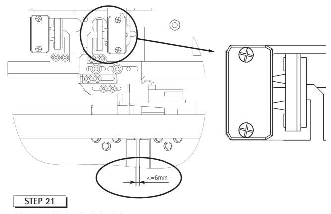
Adjust the position by using the long holes.
