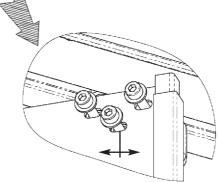
Use the long slots to adjust the panel position. For flat panel according chapter 6 or Quick Installation Guide. PM.2.002171
