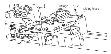
To adjust the gap between the linkage and the sliding blocks you have to adjust the vertical operator position.
